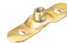
ED37 / EM37 / EH37 Top Plate For attaching sliding door carriages to timber doors. Captured nut allows door height adjustment.
