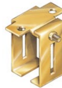
ED21 / EH21 Two Piece Bracket For tight spaces and blind pelmets. Fix one half of bracket, place track, then bolt on retaining half of bracket.
