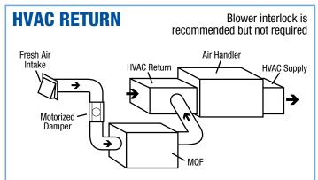
Air is brought into the dwelling through an intake wall cap and directed into the return of the HVAC system. This allows the air to be distributed faster and uses the HVAC system to "pre-condition" the air before entering the home. The HVAC fan must be operating for this to be effective.
