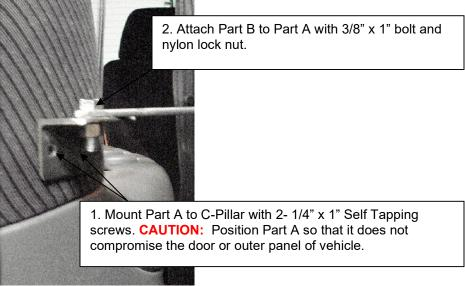
If Part B reaches the aluminum Pivot Block on the ramp attach Part B with 3/8" x 1" bolt nylon lock nut. If part B does not meet the Pivot Block completely, incorporate Part C (length may need to be shortened). Align parts B & C in the location needed and clamp with c-clamp. Mark location needed for bolt holes. Using a 3/8" drill bit - drill two holes through part C.
