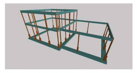
Diagram illustrating the concrete structure of the Hempro system, from the sole to the collar brace supporting the roof.
