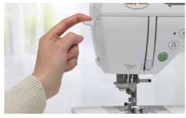
Advanced Needle Threader With just a few simple motions, your needle is threaded and ready to use - it's so easy, you can do it with one hand!
