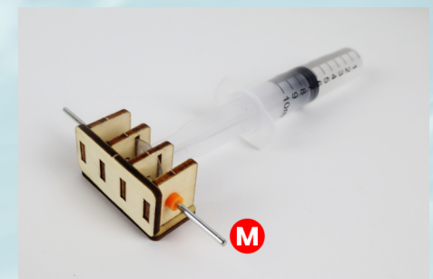
Step 4: Insert an iron rod and put orange fixing rings on each side.
