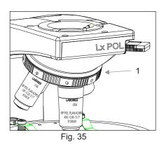
Rotate the revolving nosepiece (1) so that the objective to be used is in line above the specimen. Always use the knurled surface to rotate the objective nosepiece.
