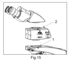
Install the observation head using the following procedure:
