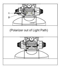
This high quality primary polarizer (1) is 360 degree rotatable with fiducial marking (2) for quick identification of Polarized / Cross Polarized positions.
