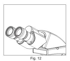
Lx POL comes with a pair of Eye Pieces. One of the eyepieces has a crosshair reticule to mark the center of the field of view and the second for normal viewing. Orientation of the Eye Piece with respect to the Polarizer and Analyzer is ensured by the eye tube lower that slides into the observation Bino Body tube. These eye pieces also have a focusing mechanism for diopter correction & foldable eye guards to prevent ambient light from entering into your line of vision.
