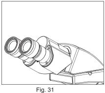
The inter-pupillary distance adjustment consists of regulating the two eyepieces to align with both eyes' pupils so that you can observe a single microscopic image through two eyepieces in stereo vision. This greatly helps to reduce fatigue and discomfort during observation.
