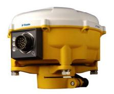
Each unit contains a GPS receiver, antenna, and isolation system all in a single housing. It is designed specifically for installation on the blade or cab for use with GCS900 3D Grade Control Systems.
