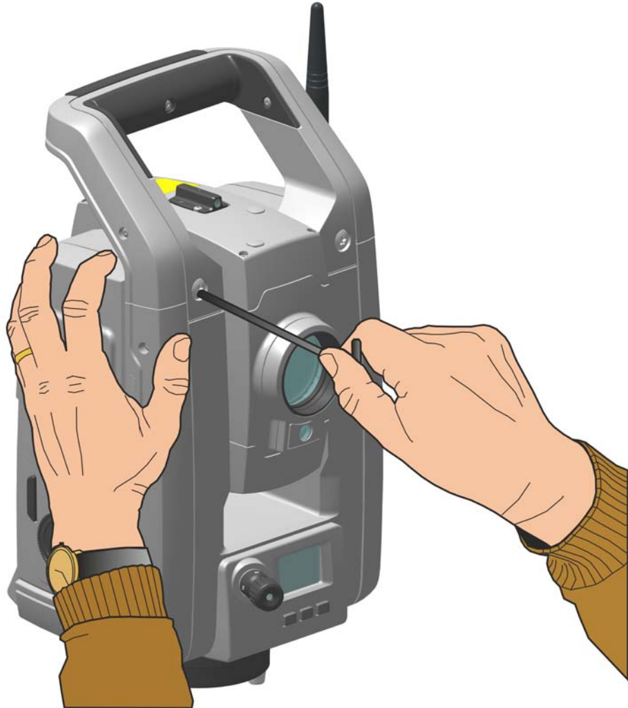
Figure 3.13 Removing the instrument handle
