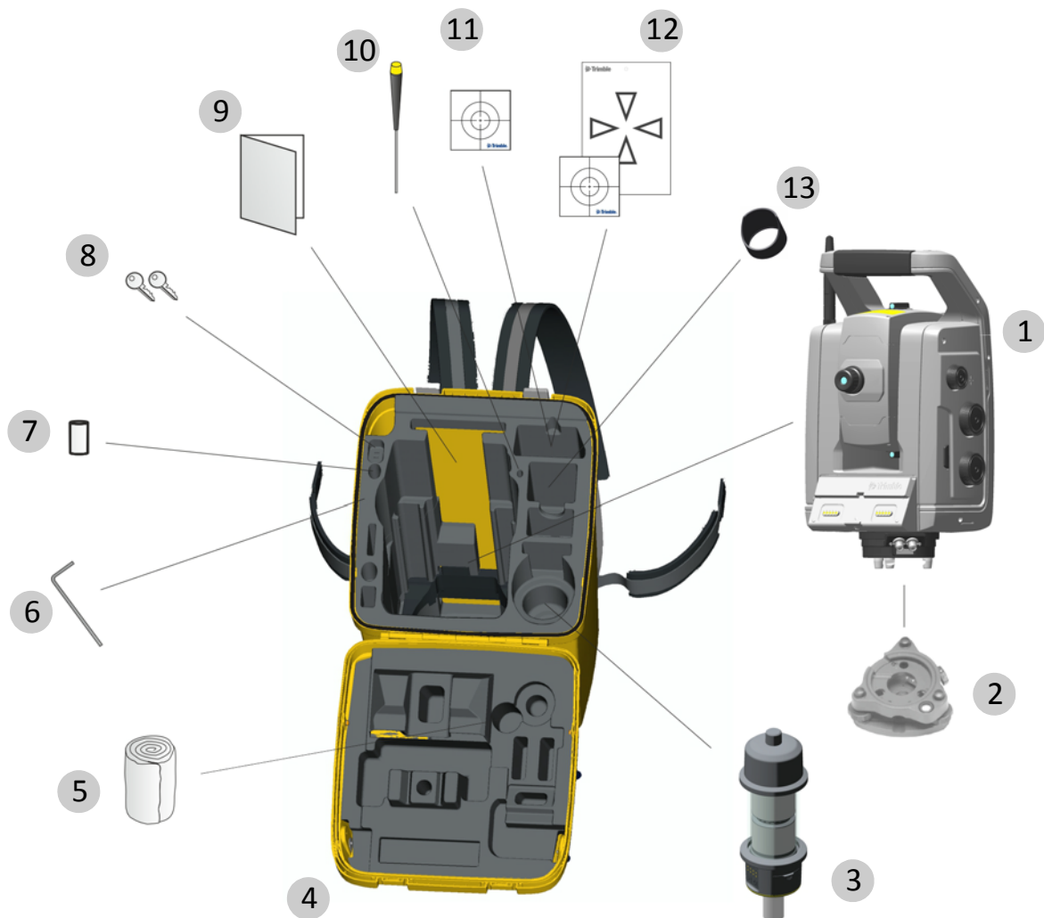
Figure 2.1 Position of items in the instrument case
