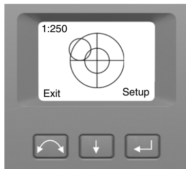
Figure 3.11 Electronic leveling screen on the face 2 display
