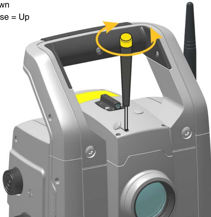
Figure 4.6 Laser pointer vertical position adjustment
