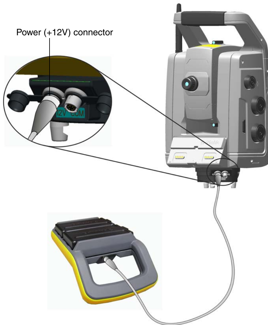
Figure 6.2 Connecting the Multi battery Adapter
