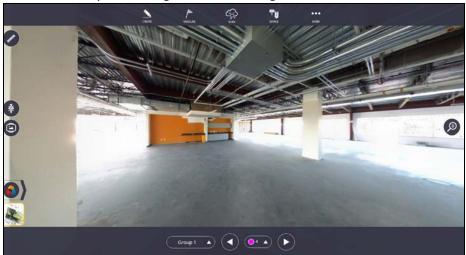
3. You can now use the View Options Ribbon to change the color of the scan. You can cycle between four options - grayscale, true color, unmeasured points, and scan intensity.
