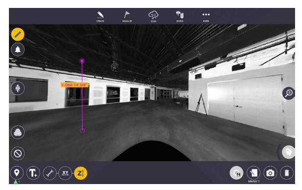
This is an example if you are using the Z-axis lock. Once you select a point on the ground or ceiling, the software will automatically follow the z-axis on your next click. The measuring tool will measure parallel distances between walls on an XY-axis lock.
