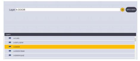
7. Now when you open the Station Manager you will see next to the station number that the scan has been assigned to a layer. When you manipulate this layer through the settings menu, this scan will be affected as well.
