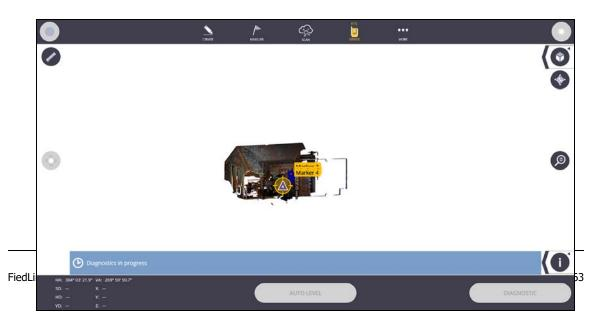
4. The diagnostics report will automatically appear once it has finished and the lights on the Trimble X7 turn green. Here you will have the option to change the file save location and file name using the **Edit** button.
