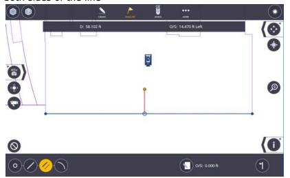
11. Tap on the first point to be measured if you entered an *Interval Distance*.
