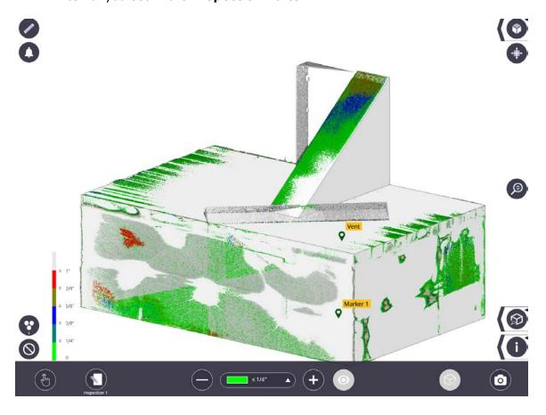
9. You can produce several model inspections with different tolerances within the same project. Simply tap More > Map to return to Map view and then go back into the Scan > Inspection menu and conduct a new inspection.
