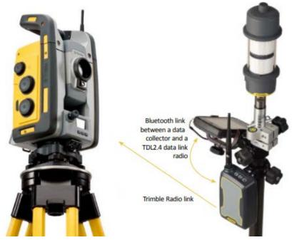
**NOTE:** When connecting to an RTS using a **Trimble Data Link Radio**, the radio must be paired before first use.
