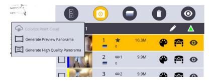
4. Once you tap on that, the art palette icon will begin to spin. This means the program is working on creating a panoramic image in the background. You can check the status of this process by tapping on the notification bell in the top left corner.
