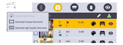
4. Once you tap on that, the art palette icon will begin to spin. This means the program is working on colorzing this point cloud in the background. You can check the status of this process by tapping on the notification bell in the top left corner.
