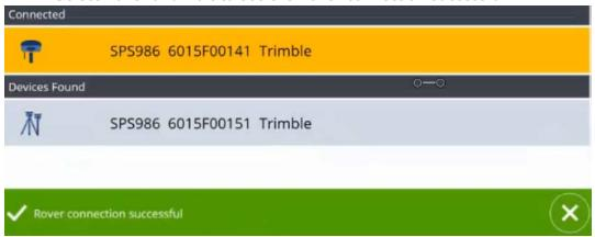
5. Once the Rover is connected and receives corrections, GPS precision will be in tolerance.
