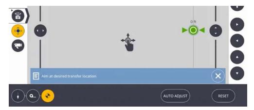
5. With the prism over the new elevation point to check for cut or fill. When aiming with the laser, move the laser to the correct vertical position and click **Auto Adjust** to move the laser to the correct elevation.
