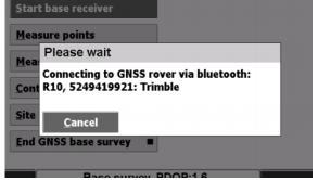
5. After the TSC3 connects to the receiver, the receiver will now look for your Base station via internal radio.
