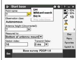
6. Add Antenna height (of receiver above the point) and where the height is Measured to (Bottom of receiver)
