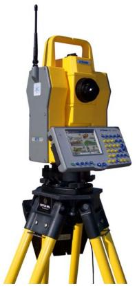
**Angle and Distance Sensor Accuracy** – The ATS is equipped with very precise angle reading systems, accurate in both horizontal and vertical to 1 arc second. The high-accuracy measurement system contributes to the 3D positioning accuracy, especially in the height component when working at longer ranges.
