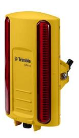
**Linear Detection** – Exact laser strike positions to within 1.5mm (0.06") for precise automatic grade control. Unlike other laser receivers that provide only 5 to 7 fixed relative grade regions, the LR4100 provides a continuous, absolute laser strike position to precisely measure the actual height deviation from "On Grade." This feature gives you the highest accuracy and grade performance.
