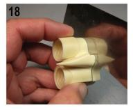
5. The kit exhaust fairing is too long (modelled on the B-1A with shorter exhaust nozzles). Shortening the exhaust fairing leaves the nacelle with an oval, rather than round, cross section. It's fairly easy to correct this.
