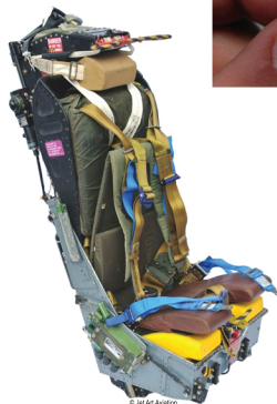
Assembled seat showing upper and lower ejection handles installed.
