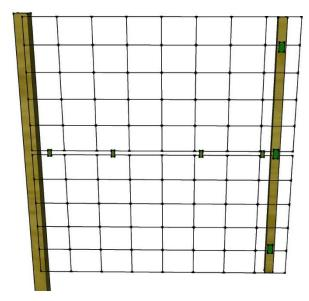
For a meter wide gate use the two panels in the same way as you would the fence panels using the joining clips and the post clips. Only this time you use the post clips the other way up and screwing them to the piece of batten provided. The batten should be placed approximately 50mm in from the end of the gate panels so that the gate panels sit flat against the second gate post.
