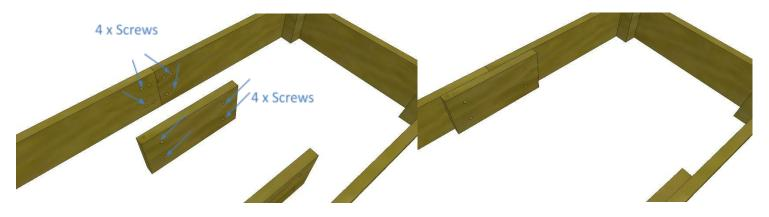
The last stage for beds larger than 6" tall then we supply vertical joiners to fix the boards layers together. This is done either in the centre of each board or in the centre of the side joiners on the 6ft or 8ft raised beds. Using screws in the holes provided.
