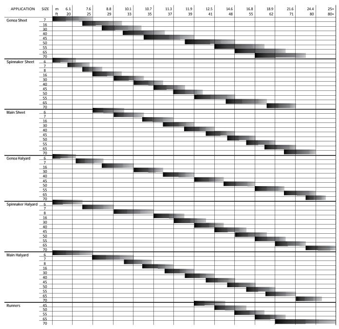
Lighter shading represents the upper limit of the model. If in doubt, move up a model.
