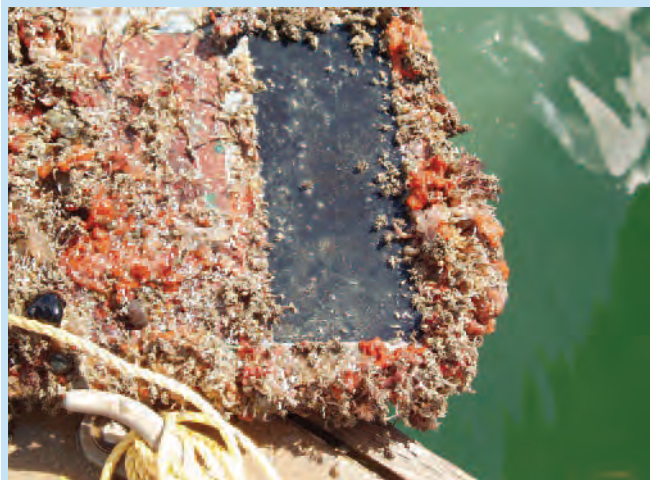
Six weeks in the BVI: The black paint on the right is Micron and the red paint on the left is not.
