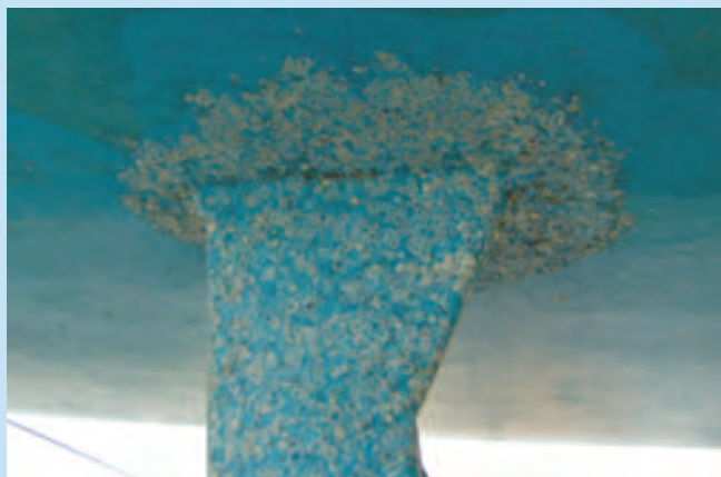
Burnback: This is caused by improperly priming the underwater metal. The copper biocide is eroded away due to electrolysis and no antifouling protection is left. This will continue on the fiberglass in concentric circles away from the metal. While this most commonly happens with paints that have an acrylic resin it can happen with any antifouling paint.
