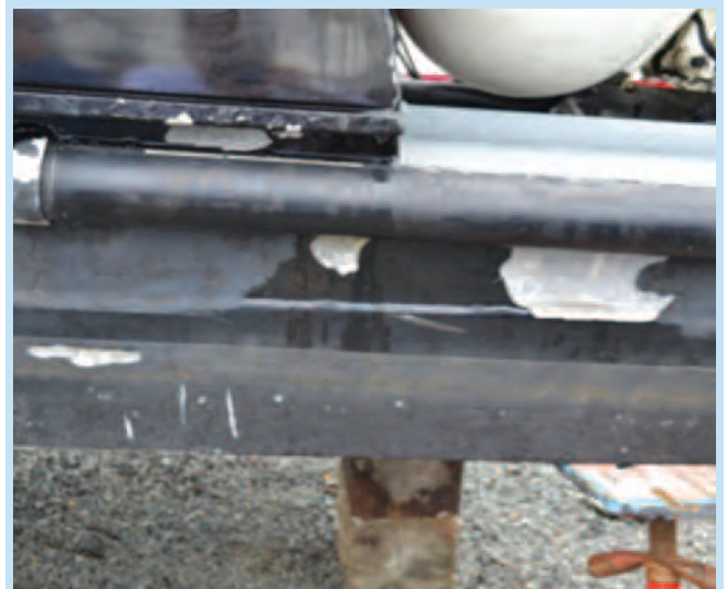
Detachment: Antifouling peeling from improperly primed aluminum.
