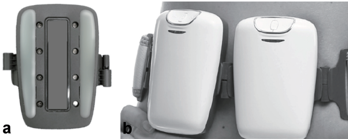
Figure 1. The Tone applicator. (a) Electrodes side of 1 unit. (b) Tone units on a belt attached to the abdomen.
