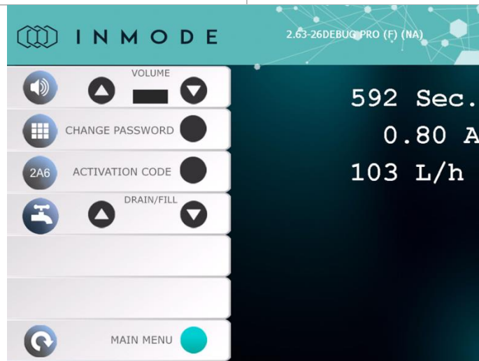
Figure 9-6: Time Counter Water Pump Current Value (right side of screen)
