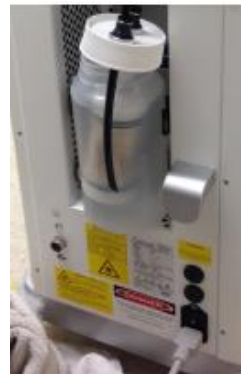
Figure 9-9: Water Bottle in Drain Position
