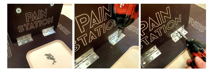
Once all the screws have been used check the movement by removing the M10 x 50 Bolts and Folding the Station forwards. Once you are sure the movement is good secure the Vertical Support in position be replacing the bolts. Take the two joining blocks plus 4 x M10 x 50 Bolts. Unfold the top section and secure with the bolts. Catch the thread by finger first then tighten using a 6 mm Allen Key. BEWARE the top section does not fall forward when you are completing this phase.
