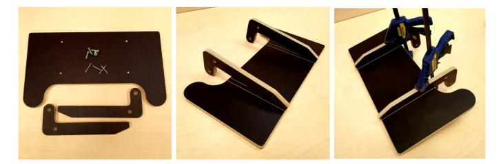
Clamp the the arms to the shelf checking that they remain within the lines. The pointed end of the arms should be flush with the straight edge of the shelf.
