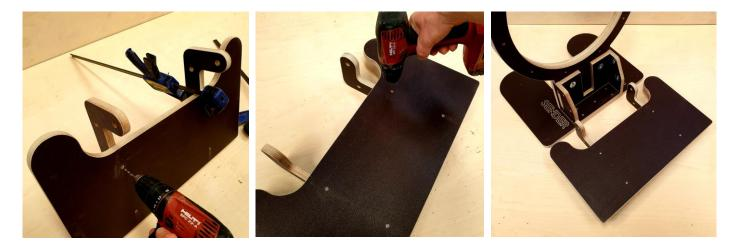
Lift the shelf into position so you can use 2 x M10 x 30 button head bolts to secure the shelf to the top two T nuts. Tighten these so there is enough movement to swing the shelf or up or down to locate the 2 lower T nut holes securing the shelf in the horizontal position.
