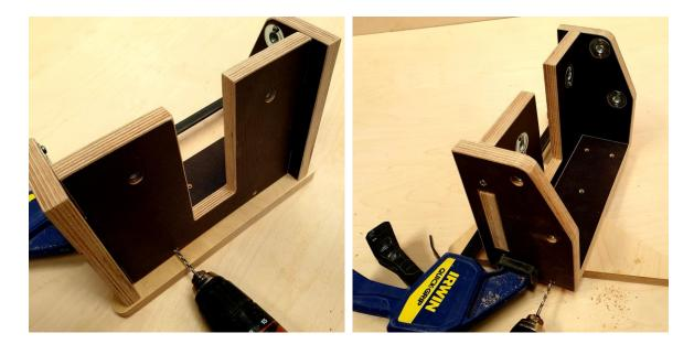
Take the structure you have made and the base plate. You will see two lines on the base plate. The structure sits equally between these lines and flush with the straight back edge as shown.
