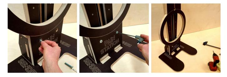
Place 2 No Hinges into the slots in front of the Vertical Support and the Base Plate. Using the 3 x 16 screws fix the hinges in place. It is important that you use the MIDDLE Hole first TOP and BOTTOM to get the best alignment!
