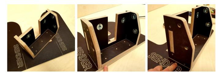
Carefully drill 25 mm through the base plate with a **3 mm** drill bit. Be careful not to drill all the way through! And into a table or floor!!!
