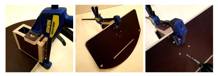
Drill through the remaining marker points ENSURING the block below has NOT moved!
