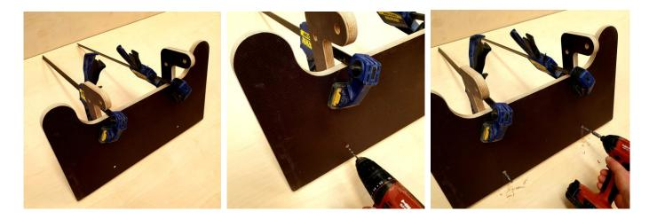
Remove one of the clamps and check that the arms remains within the lines. Drill and fix this with a TX25 screw. Remove the second clamp and repeat. The Shelf is now ready to mount to the station.
