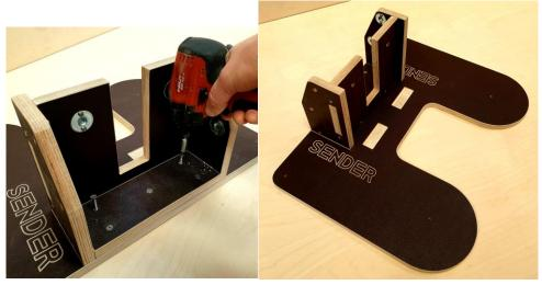
Lift the vertical support which is hinged in the middle and place this into the slot in the base plate. BEWARE of finger entrapment at the HINGE JOIN. Take 2 No M10 x 50 bolts and secure this to baseplate. When placing bolts you must always catch the thread with your fingers first! Tighten with a 6 mm allen key (On your bike Tool!)
