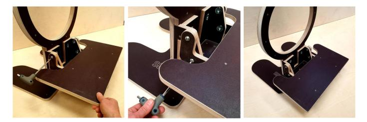
You can quickly and easily undo the bolts to remove the shelf completely. You can take out the lower bolts and swing the table up for storage OR angle the shelf down which changes the direction of airflow when using a fan. When the fan shelf is angled you will need to tighten the top bolts to create enough friction to hold the shelf in the desired position.
