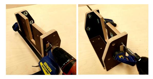
You may need to move the clamp to access some holes. Drill and fix the base block checking that it remains flush with the sides and <u>very importantly flush along the bottom</u> so it sits flat against the base plate at the next stage.
