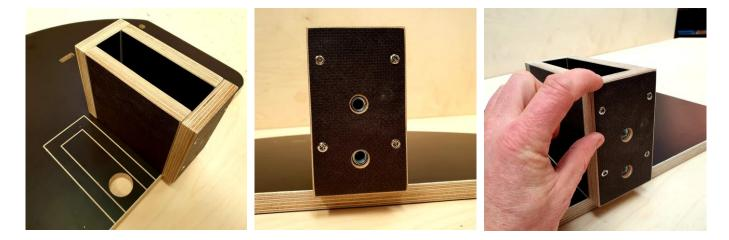
Use the adjuster block (with 2 x bolt holes) for the Table and a quick clamp to hold the components together. Adjust the block to sit within the lines. It should OVERHANG the straight back edge of table by 18 mm. You can use the remaining adjuster block (comes with the TV / Monitor mount) as a guage / guide to ensure you have 18 mm of OVERHANG. Secure this position by tightening the clamp. The Table will not pass the joining blocks on the vertical support if there is less han 18 mm!
