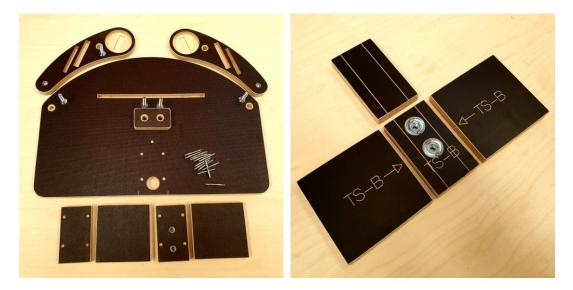
Use a Quick Clamp to hold the four components together. Adjust them until they are flush and square on all edges. Drill 50 mm through the marker points with a 4 mm drill bit and then secure with 5 x 50 TX25 screws. If you do not pre drill these holes you will split the plywood.
