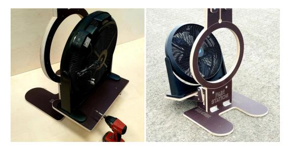
Line the front edge of the fan with the front edge of the shelf. It should be approx 3 to 4 mm back from the edge. Ensure the feet are balanced with a gap of approx 5 mm at either end. Take the two 4 x 20 Combi Head screws and secure the base to the shelf. It will help if you tilt the fan to alow better access for the drill. You may need batteries for the Fan Remote Control.
