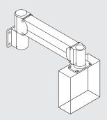
The mounting surface supports the arm and the enclosure is suspended from the arm. This is the most popular configuration.
