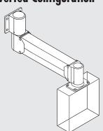
The mounting end is inverted, resulting in the arm being suspended from the mounting surface. Inverted post-mounted arms are popular for supporting the arm from the ceiling.
