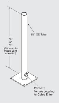
For use with a post top mount Vertica arm, the floorpost is a very popular method of mounting an arm when a structural surface is not available. The 74" post is for Vertica arms and the 79" post is for Vertica arms with a middle joint extension. Fabricated from heavy wall  $3\frac{1}{2}$ " structural tube welded to a 12" x 12" x 3/8" thick baseplate. A  $1\frac{1}{2}$ " female NPT coupling near the base for cable entry, additional couplings can be specified or located differently.
