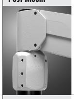
A Post Mount Vertica Arm attaches to a plain end 3½" OD tube or 3" pipe. Collar slides over post and is leveled with set screws. A pilot hole in the collar for drilling through the post and installing a 5/16" bolt is provided. Cables enter through post (optional posts have 1½" NPT female coupling). Rotational Stops at 330° (±165°) are standard; alternate stops can be specified.
