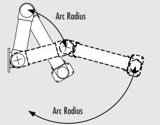
The middle joint extension adds a third pivot to the Vertica arm for in/out adjustability.
