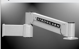
Typically used when there is a mounting surface available but not in the ideal location. The rigid wall mount essentially moves the mounting surface. Both length and angle can be specified. These extensions are preferable over horizontal and middle joint extensions for applications that require a long reach.
