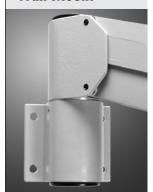
A Wall Mount Vertica Arm attaches to a vertical surface with a thru-hole pattern (4) 0.53 Ø. Cables enter through the center of mounting surface or female 2½" NPT access cap opening. Rotational stops at 180° (±90°) are standard; alternate stops can be specified.
