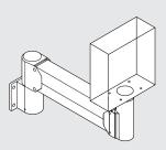
The mounting surface is supporting the arm and the enclosure is supported by the arm. A vertical extension is required for this configuration so that the arm does not come in contact with the enclosure when it is lowered and rotated. The minimum length of the extension depends on the size of the enclosure. This configuration is popular for supporting devices other than operator interface enclosures.
