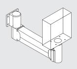
The mounting end is inverted and the enclosure is supported by the arm. A vertical extension is required for this configuration so that the arm does not come in contact with the enclosure when it is lowered and rotated. The minimum length of the extension depends on the size of the enclosure. This configuration is popular for supporting devices other than operator interface enclosures.
