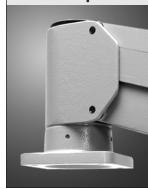
A Machine Top mount Vertica Arm attaches to a horizontal surface with thru-hole pattern (4)  $0.38 \varnothing$ . Cables enter through center of mounting surface. Rotational stops at  $330^{\circ}$  ( $\pm 165^{\circ}$ ) are standard; alternate stops can be specified.
