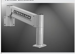
The vertical extension increases the distance between the mounting surface and the enclosure by "H". Select from standards of 4", 8", 12" or specify the exact length. Very long vertical extensions are not recommended due to the increase in the twisting moment on the arm. Generally, the shorter the better and not longer than 18".
