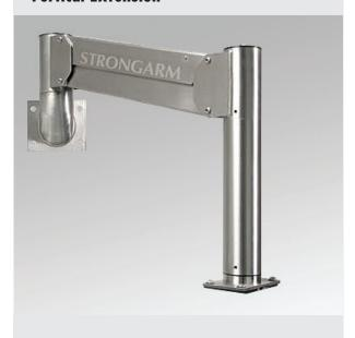
The vertical extension increases the distance between the mounting surface and the enclosure by "H". Select from standards of 4", 8", 12" or specify the exact length. Very long vertical extensions are not recommended due to the increase in the twisting moment on the arm. Generally, the shorter the better and not longer than 18".
