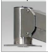
A Machine Top mount Vertica Arm attaches to a horizontal surface with thru-hole pattern (4) 0.38  $\varnothing$ . Cables enter through center of mounting surface. Rotational stops at 330° ( $\pm 165$ °) are standard; alternate stops can be specified.
