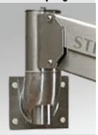
A Wall Mount Vertica Arm attaches to a vertical surface with a thru-hole pattern (4) 0.53  $\oslash$ . Cables enter through the center of mounting surface or the additional  $1\frac{1}{2}$ " NPT coupling. Rotational stops at  $180^{\circ}$  ( $\pm 90^{\circ}$ ) are standard; alternate stops can be specified.
