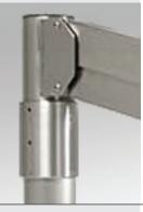
A Post Mount Vertica Arm attaches to a plain end  $3\frac{1}{2}$ " OD tube or 3" pipe. Collar slides over post and is leveled with set screws. A pilot hole in the collar for drilling through the post and installing a 5/16" bolt is provided. Cables enter through post (optional posts have  $1\frac{1}{2}$ " NPT female coupling). Rotational Stops at  $330^{\circ}$  ( $\pm 165^{\circ}$ ) are standard; alternate stops can be specified.
