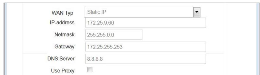
The screenshot shows the 'WAN Settings' page with 'WAN Type' set to 'Static IP'. The 'IP-address' field contains '172.25.9.60', 'Netmask' is '255.255.0.0', 'Gateway' is '172.25.255.253', and 'DNS Server' is '8.8.8.8'. The 'Use Proxy' checkbox is unchecked. Navigation buttons include '<< Previous', 'Next >>', and 'Cancel'.
