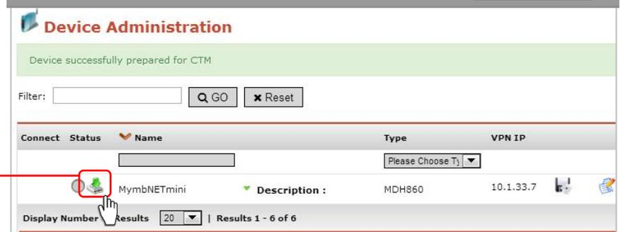
By clicking on this symbol the data saved in the CTM are shown. The configuration can still be deleted from the CTM.
