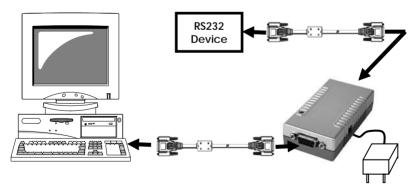
3. Connect the 5V AC Adapter or USB-to-Power-DC-Jack Conversion Cable
