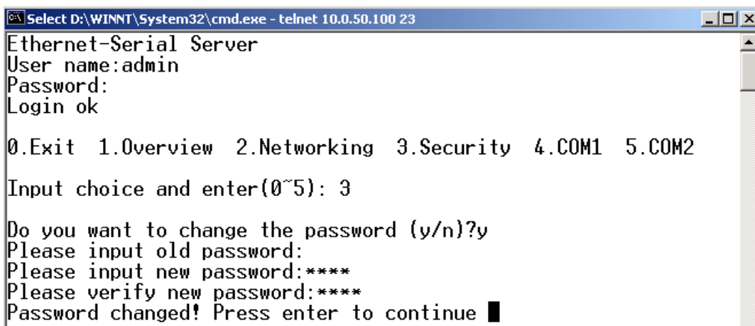
Fig. 13. changing password using Telnet
