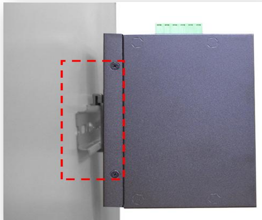
Figure 3.3 Stable the Switch on DIN-Rail
