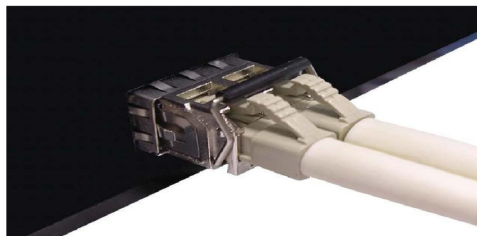
Figure 2.11 LC Connector to the Transceiver
