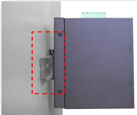
Figure 3.3 Stable the Switch on DIN-Rail
