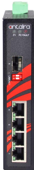
Figure 2.2 The Front Panel of LNX-0501G-SFP Series
