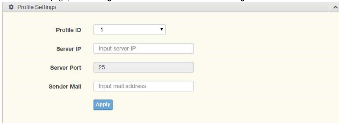
Figure 4.97 Management > SMTP Client > Profile Settings > Profile Settings
