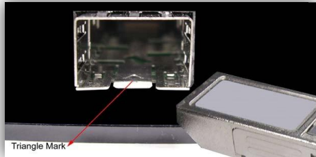
Figure 2.7 - Transceiver to the SFP Module
