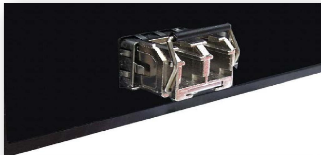
Figure 2.9 - Transceiver to the SFP Module
