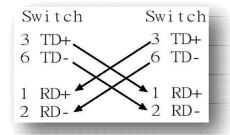
Figure 2.5 Crossover Cables Schematic
