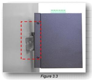
Stable the Switch on DIN-Rail
