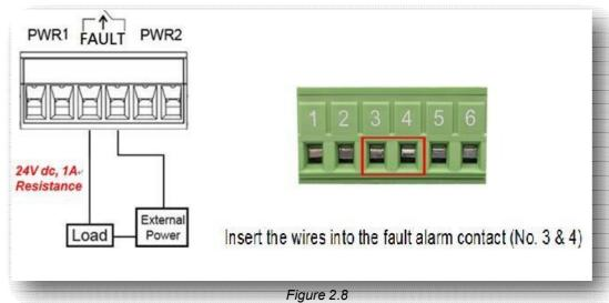
Wiring the Fault Alarm Contact
