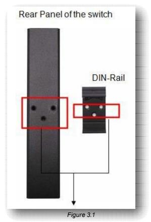
The Rear Side of the Switch and DIN-Rail Bracket
