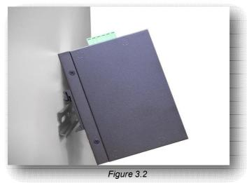
Insert the Switch on the DIN-Rail
