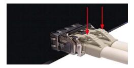
Figure 2.8 - Remove LC Connector
