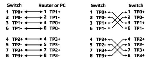
Figure 2.3 Straight-Through Cables Schematic
