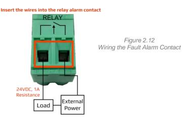
Note • The wire gauge for the terminal block should range between 12 ~ 24 AWG
