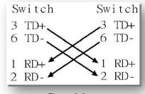
Figure 2.5 Crossover Cable Schematic
