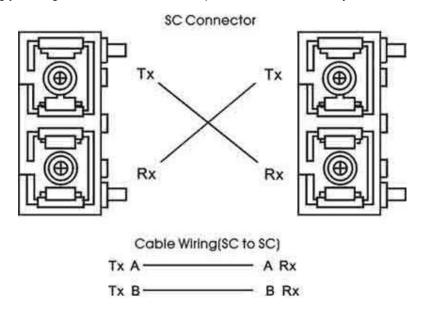
Figure 2.6 - Fiber Ports Connection
