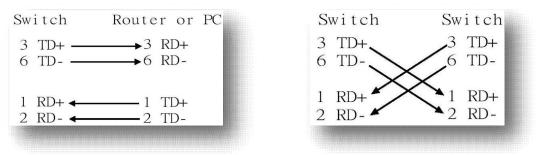
Figure 2.4 Straight-Through Cable Schematic
