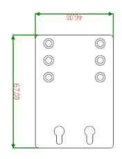
Figure 3.5 Wall Mounting Bracket Dimensions
