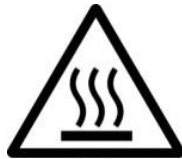
Figure 1.2 - Hot Surface Warning Label
