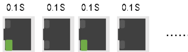
Figure 2.5 - PoE Over Current LED Sequence
