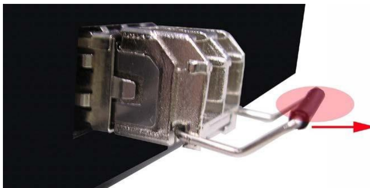
Figure 2.11 Pull Out from the SFP Module
