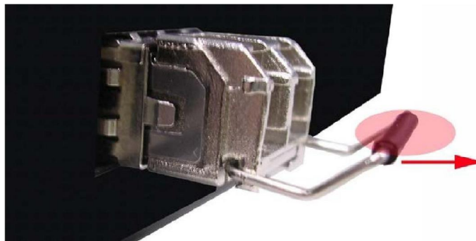
Figure 2.10 Pull Out from the SFP Module
