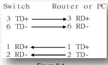
Figure 2.4 Straight-Through Cable Schematic
