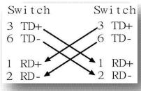
Figure 2.5 Crossover Cable Schematic
