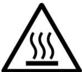
Figure 1.2 - Hot Surface Warning Label
