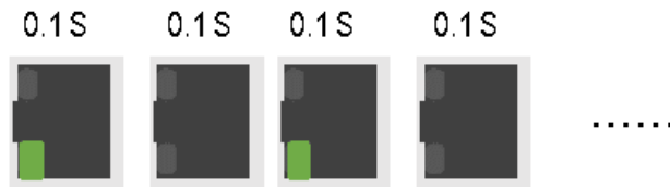
Figure 2.6 - PoE Over Current LED Sequence
