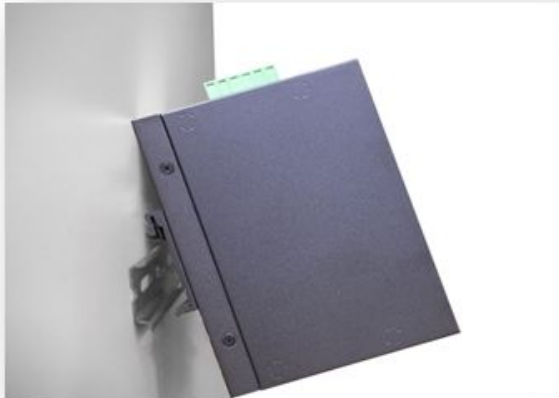
Figure 3.2 - Insert the Switch on the DIN-Rail
