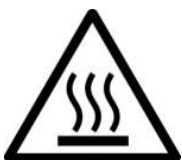
Figure 1.2 - Hot Surface Warning Label
