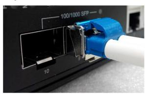
Figure 2.9 - LC Connector to the Transceiver
