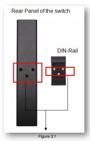
The Rear Side of the Media Converter and DIN-Rail Bracket
