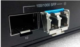
Figure 2.7 - Transceiver to the SFP Slot
