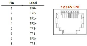
Figure 2.4: RJ-45 Ethernet Port Pin
