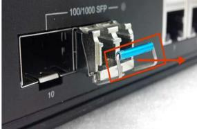
Figure 2.10 – Remove LC Connector
