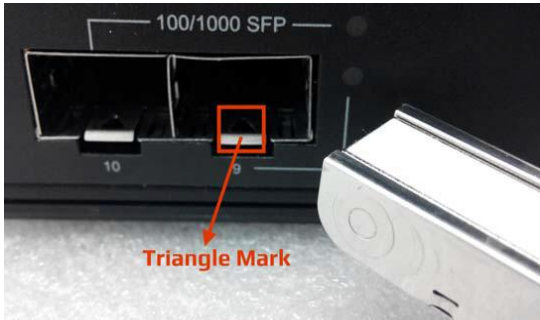
Figure 2.6 - Transceiver to the SFP Slot
