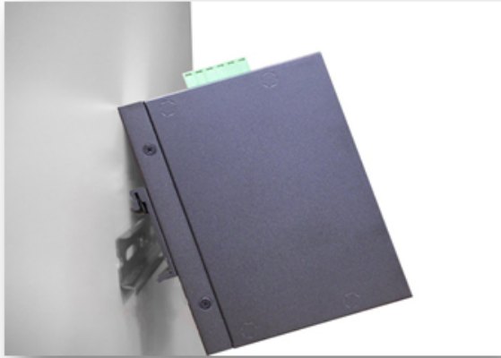
Figure 3.2 - Insert the Switch on the DIN-Rail
