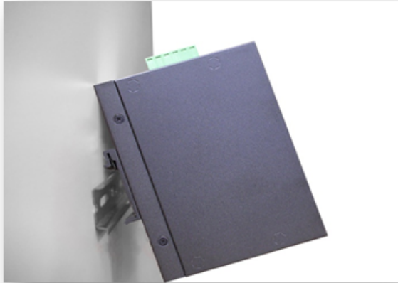
Figure 3.2 - Insert the Switch on the DIN-Rail
